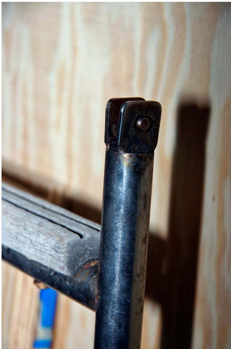
Detail of pin and pivot point.
