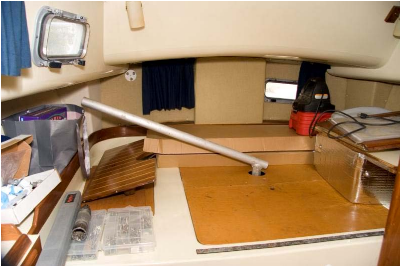
Emergency Tiller in Place (positioned 90 degrees off for clearance port & stbd)
